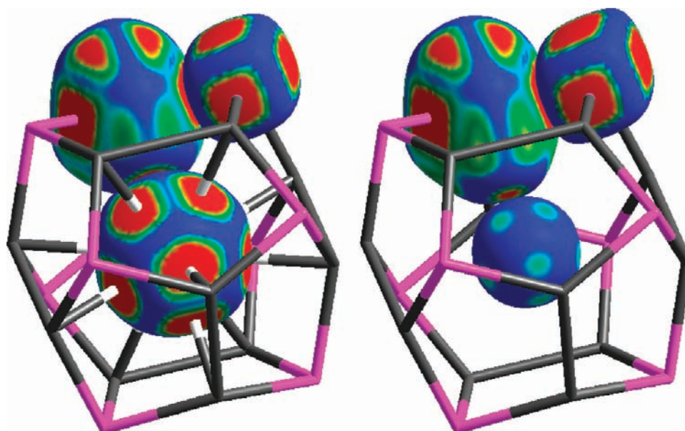
Figure 8. (a) Atomic Hirshfeld surfaces of La (white), Co (magenta), and Sb (gray) in the partial La-filled skutterudite \text{CoSb}_3 . (b) Atomic Hirshfeld surface of a Xe atom in \text{CoSb}_3 .
